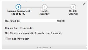
The Assembly Open Progress indicator provides details about the status of the three main operations that run while you open an assembly or drawing. These are opening (loading) the components, updating the assembly/drawing, and finally updating and repainting the graphics. Determining which of the operations take more time while opening your assembly or drawing could indicate a potential area of your design, where to port modifications for performance improvements.
