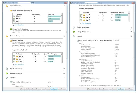
The **Performance Evaluation** displays information about how your assembly or drawing is performing. This analysis includes open performance, rebuild performance, and display performance of the models in your assembly. The evaluation also displays the settings performance, highlighting particular options to improve the file performance. Furthermore, it provides statistics about the referenced parts and subassemblies within the top-level assembly.
