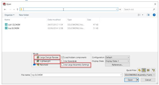
Lightweight mode loads a subset of data from assembly files. This data includes the 3D body data, mates, and reference geometry. For the vast majority of assemblies, Lightweight is the best choice of assembly modes, limiting the initial amount of data in transit and in memory when opening and beginning to work within a larger assembly or drawing. In Lightweight mode, you can add mates, create assembly features, calculate interference detection, add annotations, evaluate measures, and more.
