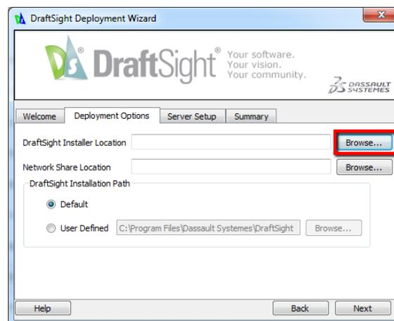
7. Add the Network Share Location by selecting **Browse**. The deployment package will be created in this location. The location must be accessible to client machines.
